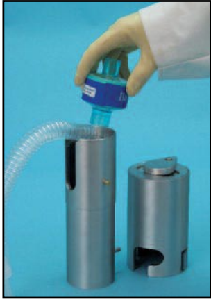
1 Insert Venti-Scan™ IV Kit in canister
