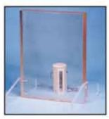
The Bench Top Shield for gamma radiation is constructed of 1.375" thick (35 mm) lead acrylic, providing the equivalent of 0.060" (1.5 mm) lead for shielding gamma radiation. Lead acrylic can be used with low-energy gamma emitters. Lead acrylic is not recommended for beta emitters. This lightweight, sturdy shield is ideal for use in hoods, on labo-
