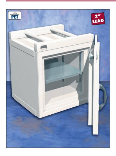
Conveniently loaded from the front, this Storage Safe is ideal for storing large quantities of high activity radioisotopes. Shielded with a thickness of 2" of lead, the safe is encased in a powder-coated steel jacket and features an adjustable shelf. The lead-lined door is hung with heavy duty non-sagging hinges and is key-locked to prevent unauthorized access.
