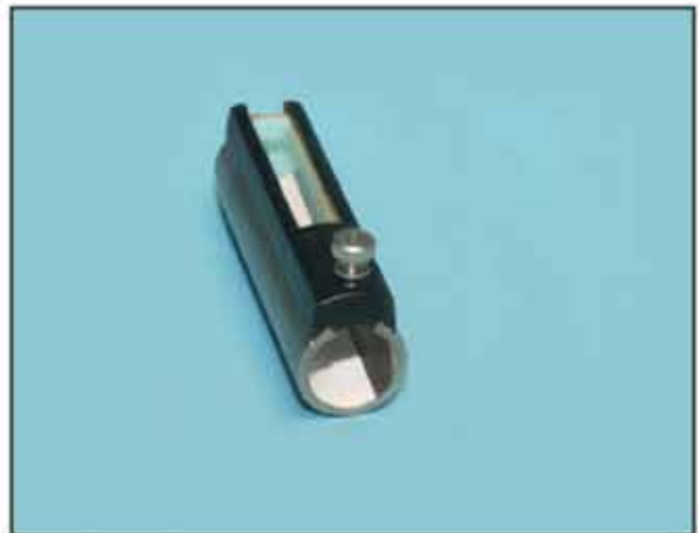
A thumbscrew holds syringe firmly in place.
