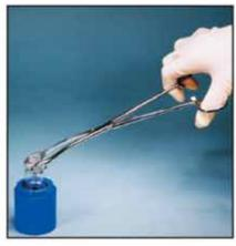
Surgical forceps are excellent handling devices for small items in the hot lab. No need to physically touch vials, ampules, etc. Forceps are made of surgical grade steel.
