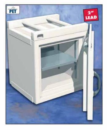
Conveniently loaded from the front, this Storage Safe is ideal for storing large quantities of high-activity radioisotopes. Shielded with a thickness of 2" of lead, the safe is encased in a powder-coated steel jacket and features an adjustable shelf. The lead-lined door is hung with heavy duty non-sagging hinges and is key-locked to prevent unauthorized access.
